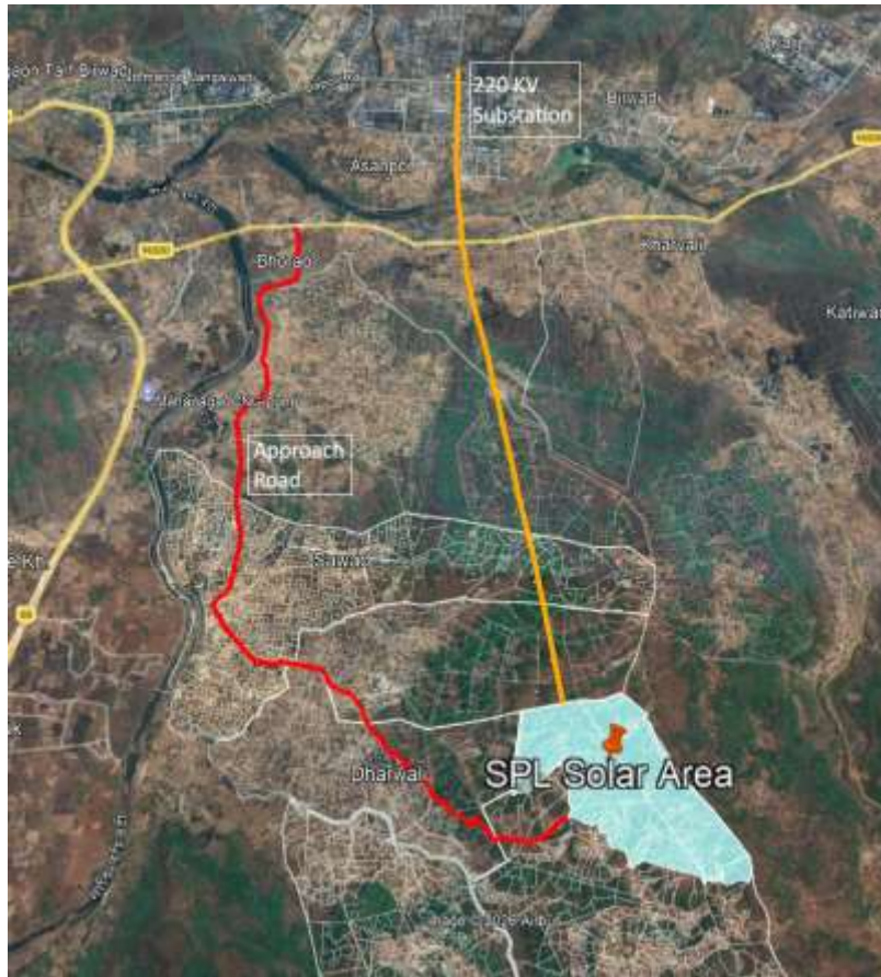
Solar Plant of 150 MWp near Mahad
